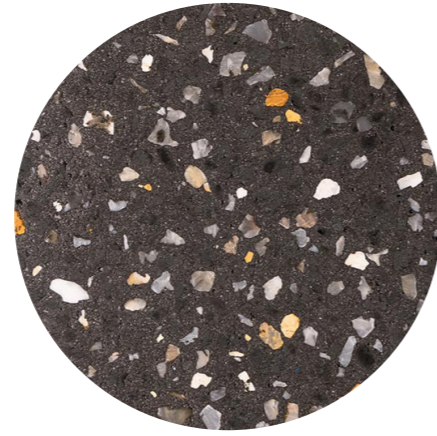
E.CON-02 HONED CONCRETE FINISH
