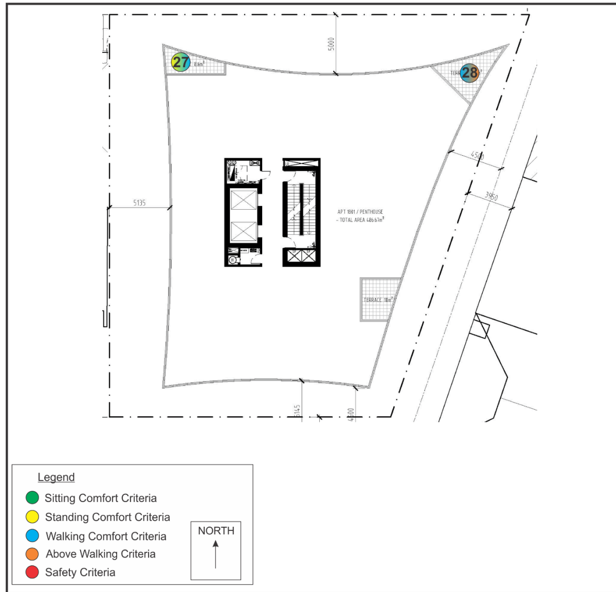
Figure 10 – Summary of level 18 wind conditions for the Proposed Configuration for 360° of wind direction
