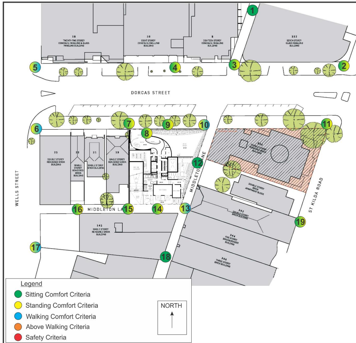
Figure 7b – Summary of ground level wind conditions for the Proposed Configuration for 360° of wind direction.
