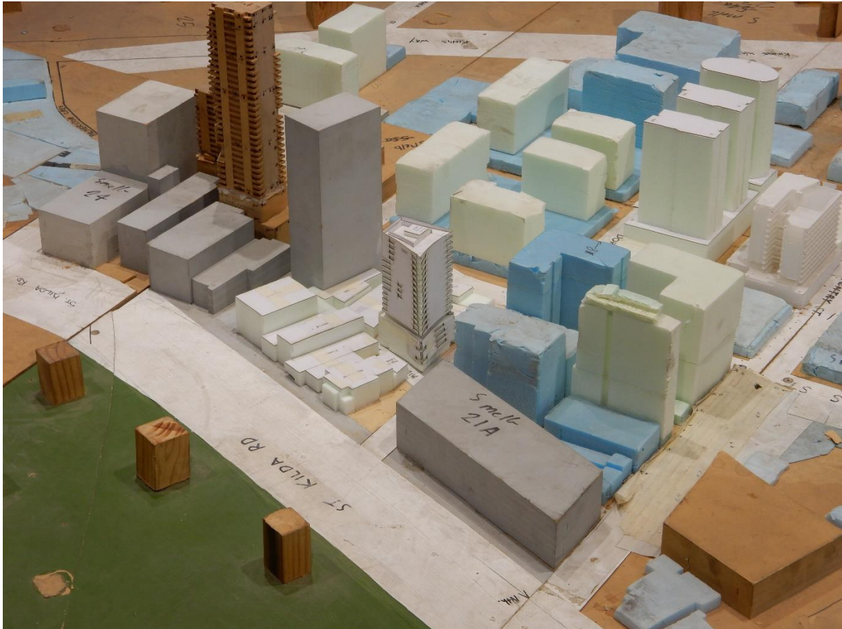
Figure 5 – View from the northeast of the 1/400 scale model of the 11-17 Dorcas Street Development in the wind tunnel.
