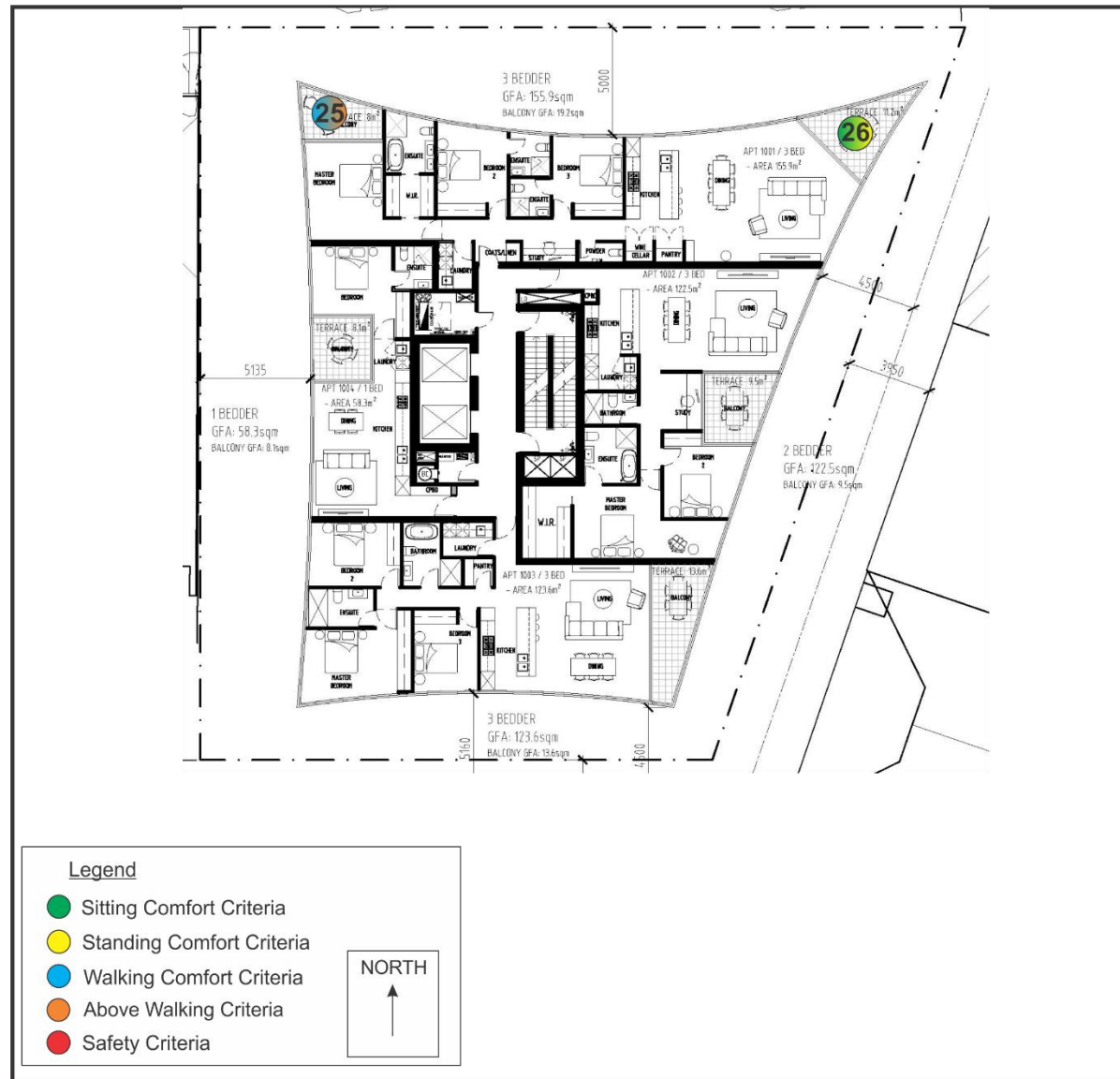
Figure 9 – Summary of level 11 wind conditions for the Proposed Configuration for 360° of wind direction
