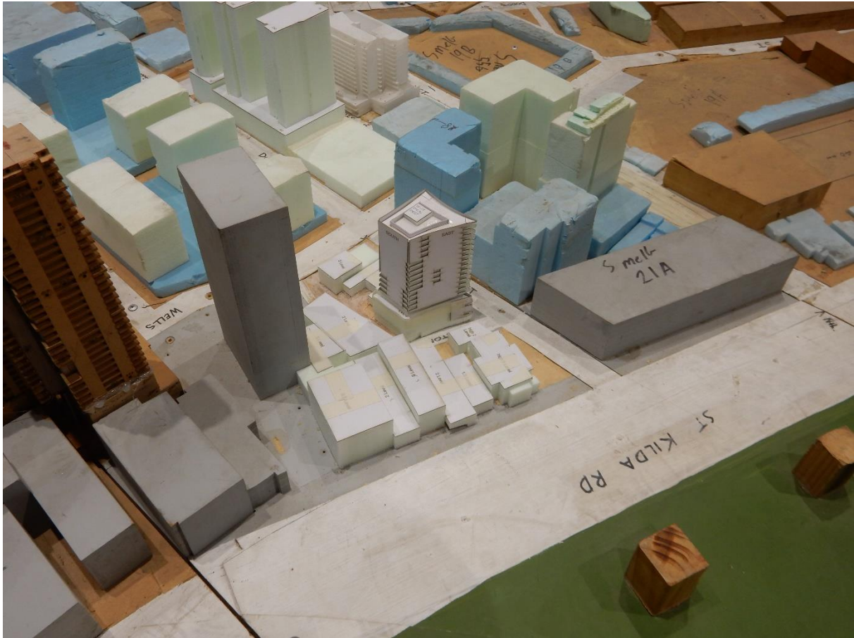
Figure 4 – View from the southeast of the 1/400 scale model of the 11-17 Dorcas Street Development in the wind tunnel.
