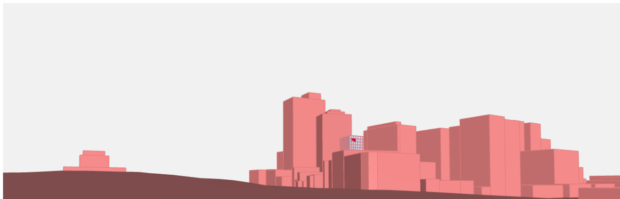
Figure 7: Representative perspective. Glare points exceeding the limit are shown in red (April and August 5pm).
