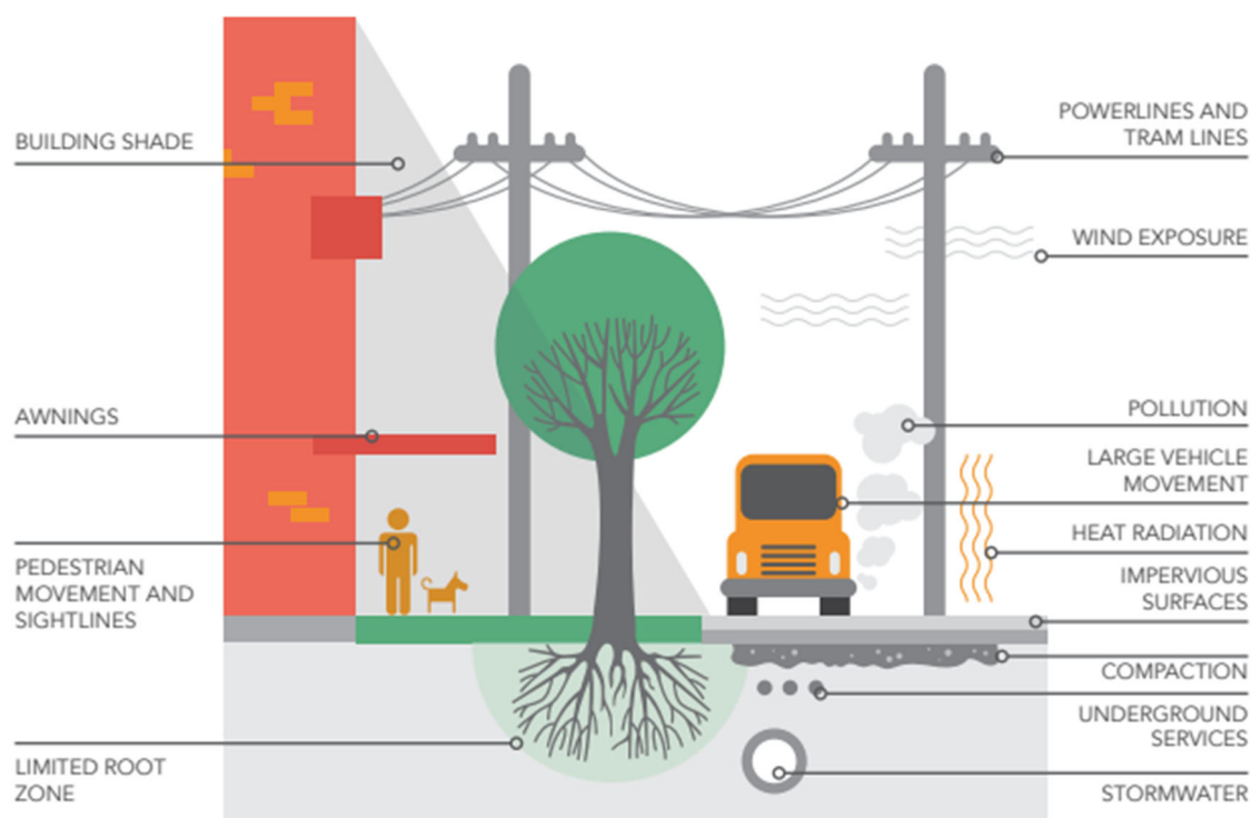
Figure 7. Illustration of common constraints for trees in urban areas. Source: Maribyrnong City Council (2018) Urban Forest Strategy .
