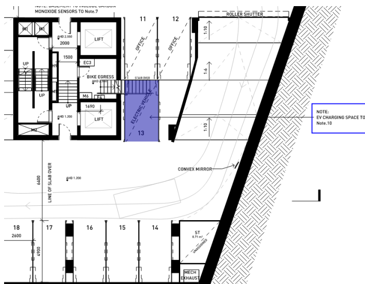
EV charging located in Basement 01
