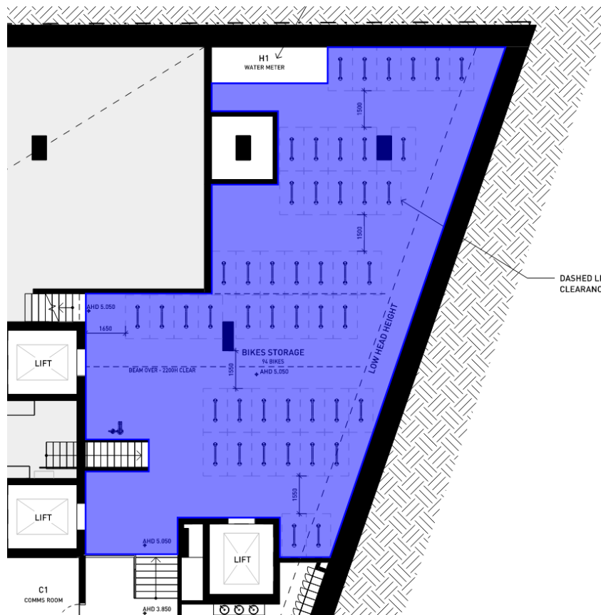
Bike Storage located in Basement Mezzanine
