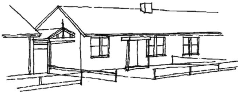
This carport, although setback by 500mm, has uncharacteristic decoration making it a prominent element of the site in comparison with the dwelling, thus attracting attention not warranted by a secondary element
