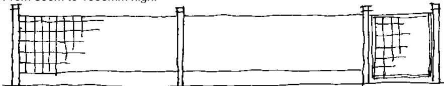
Modern weld-mesh fixed to either a galvanised steel or timber frame. 1000mm high.
