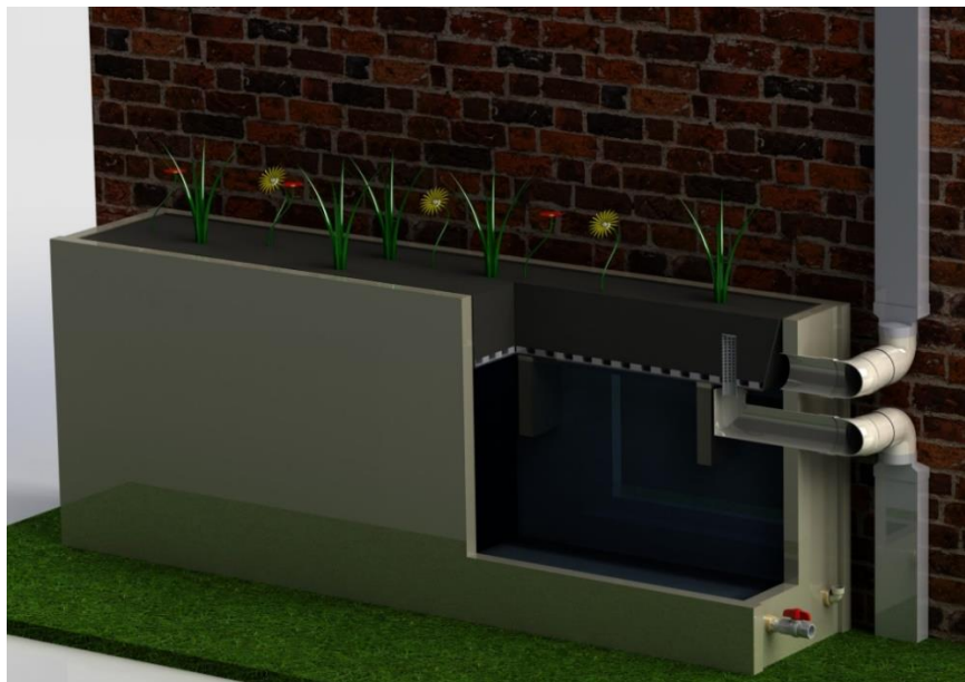
Figure 3.2 Typical Raingarden in ground illustration
