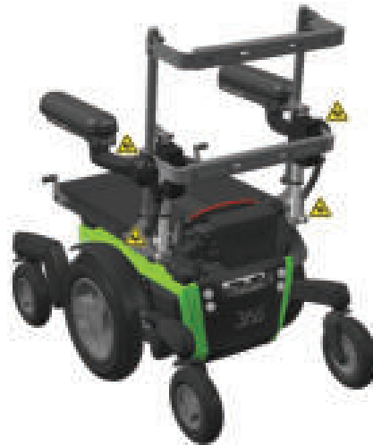
Figure 4.3a Fold Forward grab handle
