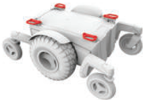
Figure 5.2a Magic 360 lifting points
