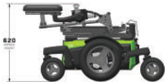
Figure 4.3b Magic 360 Fold Forward height
