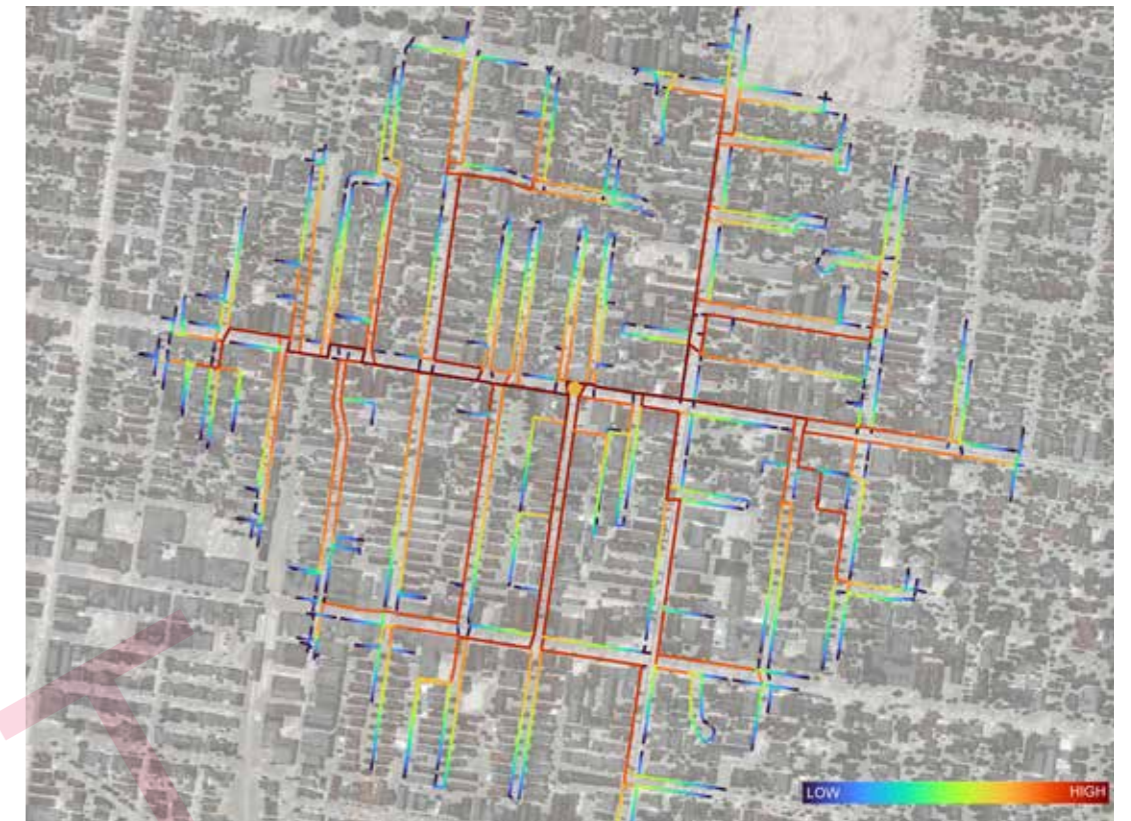
Figure 12 (above): Pedestrian route usage density for Inkerman Street with a maximum direct sun exposure limit of 10 minutes, simulated for December 22nd at 3:30 pm. The colour spectrum ranges from red, represent streets with higher pedestrian traffic density, through to dark blue, indicate routes with lower usage.
