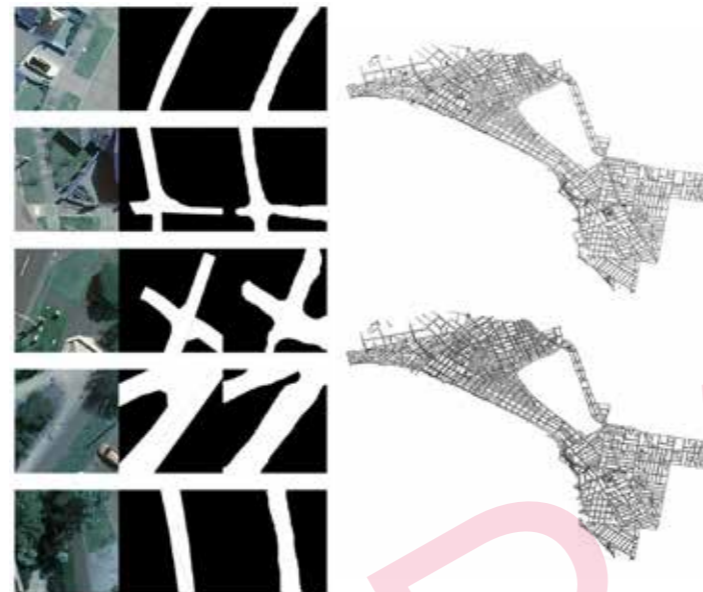
Figure 1: above, examples of the mask output from the best performing fine-tuning model. The model is pre-trained as the backbone of DINO-MCina self-supervised manner and then fine-tuned on footpath segmentation task training set with 1000 remote sensing images. Right, visualisation of the whole generated network with top right image of the ground truth footpath network, and bottom right showing the generated footpath network using our pipeline (Wanyan et al. 2023).
