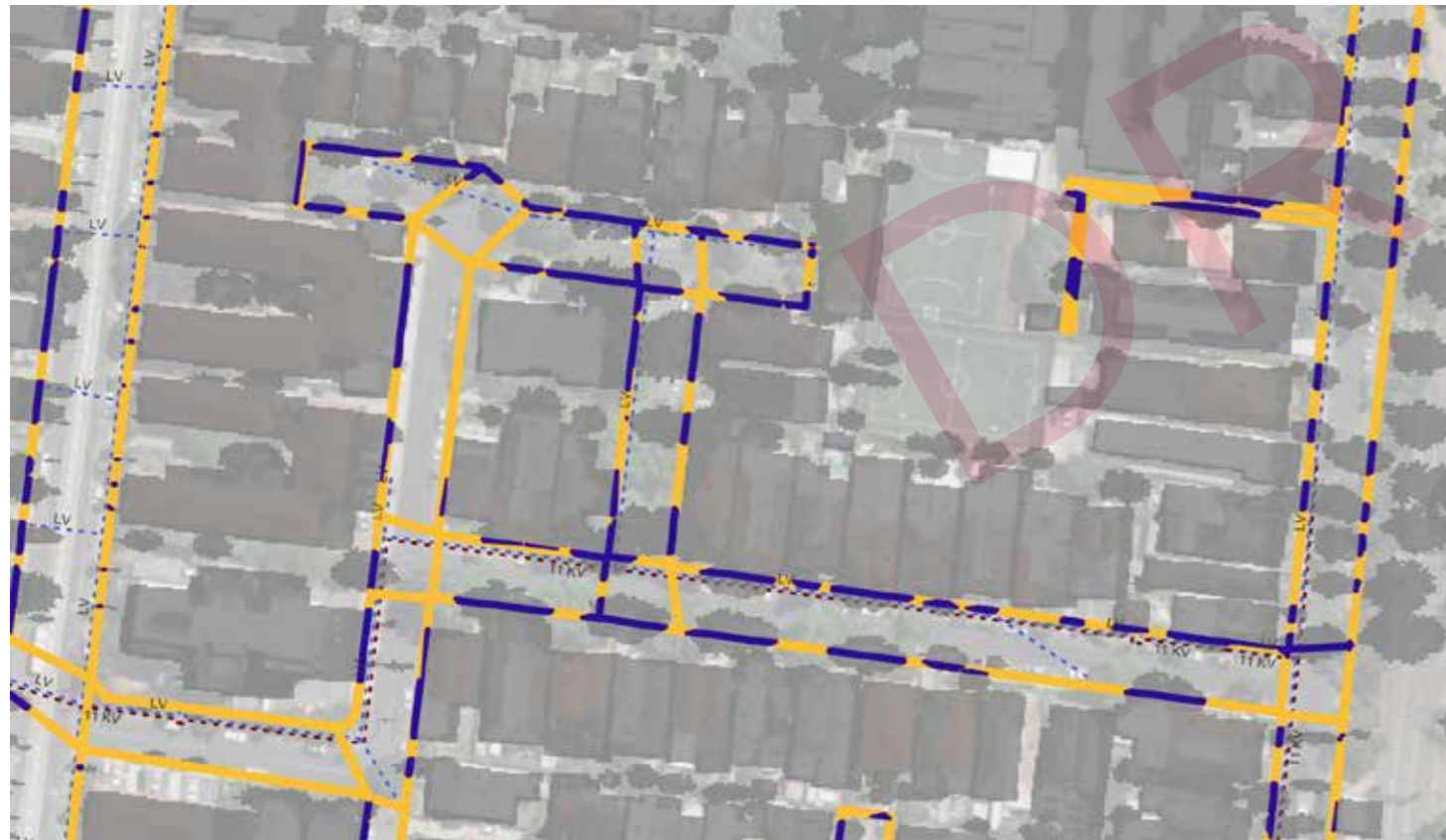
Figure 9 (below): Detailed plan view showing 3.30pm December 22 intersected with footpath vector data with yellow footpath areas show footpath that is fully in shade, blue shows footpaths in shadow, with dotted lines showing overhead powerline dataset.
