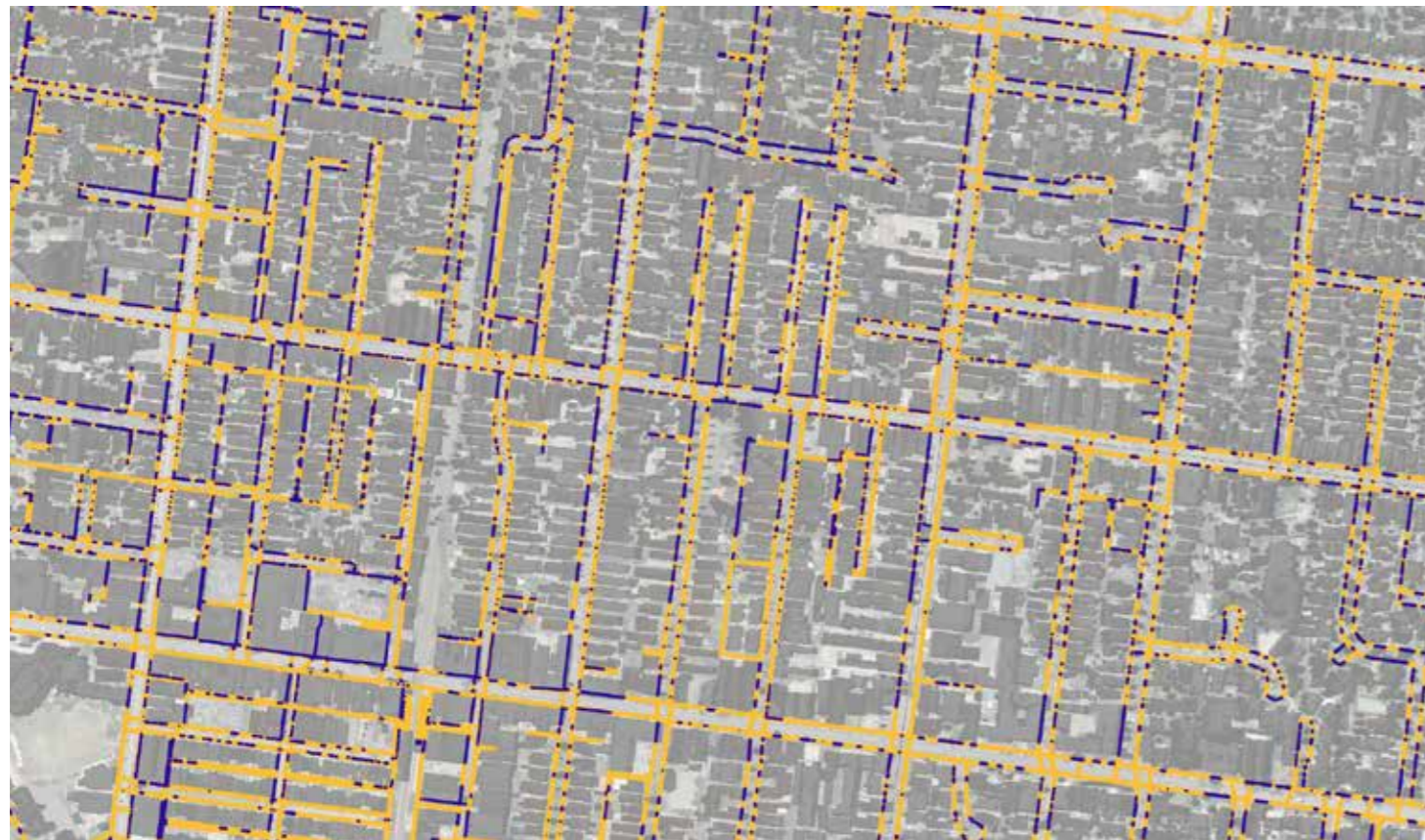
Figure 8 (above): Down-scaled shadow map calculated for 3.30pm December 22 intersected with footpath vector data. Yellow footpath areas show footpath that is fully in shade, blue shows footpaths in shadow.
