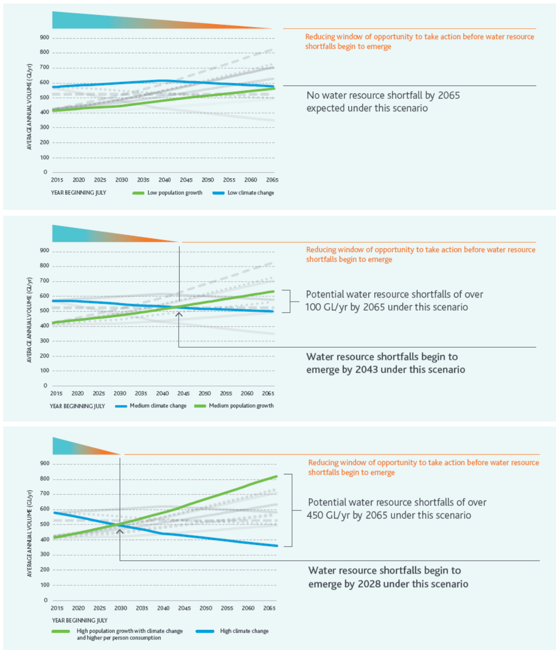
Figure 31: Three key scenarios of supply and demand used during the development of the Melbourne Water System Strategy (2017) this strategy: low change scenario (top), incremental change scenario (middle), and rapid change scenario (bottom) 50
