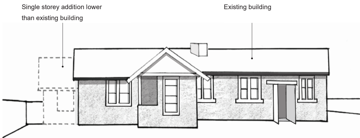
Figure 14. A simple gable side addition, possible where there can be a boundary setback.
