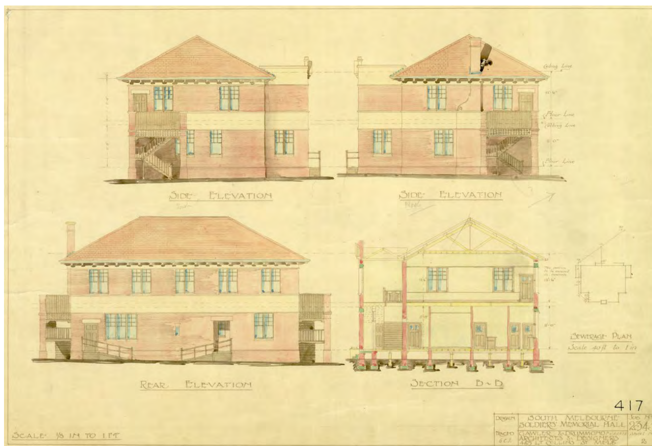
Figure 14. South Melbourne Soldiers' Memorial Hall elevations and section, Gawler and Drummond, c.1924. Note the simpler external staircases, with timber balustrades and latticework instead of masonry arches (City of Port Phillip Collection)
