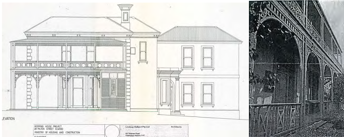
Figure 3: At left, building plans showing the reconstructed verandah (Source: Ravelston Council File) and, at right, an image of the verandah c. 1985 (Source: Bick, 1985)
