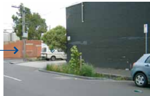
Figure 29. Medians and vegetated road verges can be retrofitted to accept stormwater for treatment.
