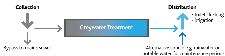
Figure 10. Schematic of greywater reuse system
