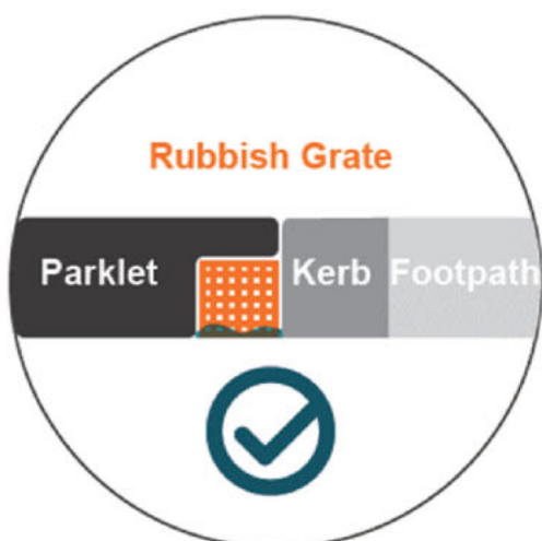
Figure x: A rubbish grate will prevent litter from being trapped under the platform.
