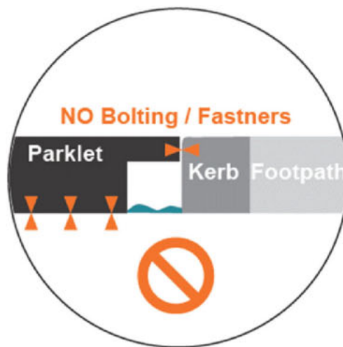
Figure x: Structures must not be fixed to the pavement or the kerb upstands.
