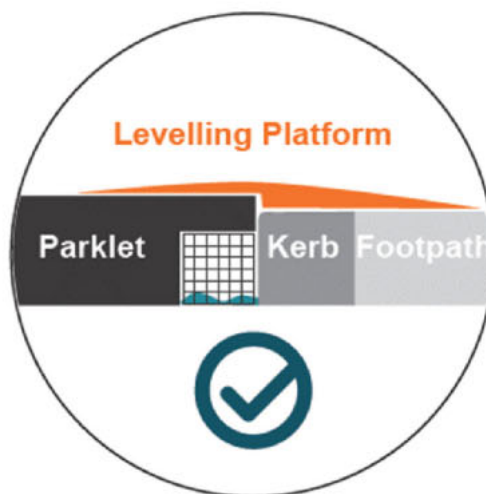
Figure x: Leveling platform creates a smooth transition and prevents tripping hazards.
