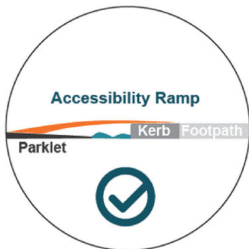
Figure X: Seasonal Business Parklets are not required to have a platform that is level with the footpath and may therefore use a ramp onto the carriageway.
