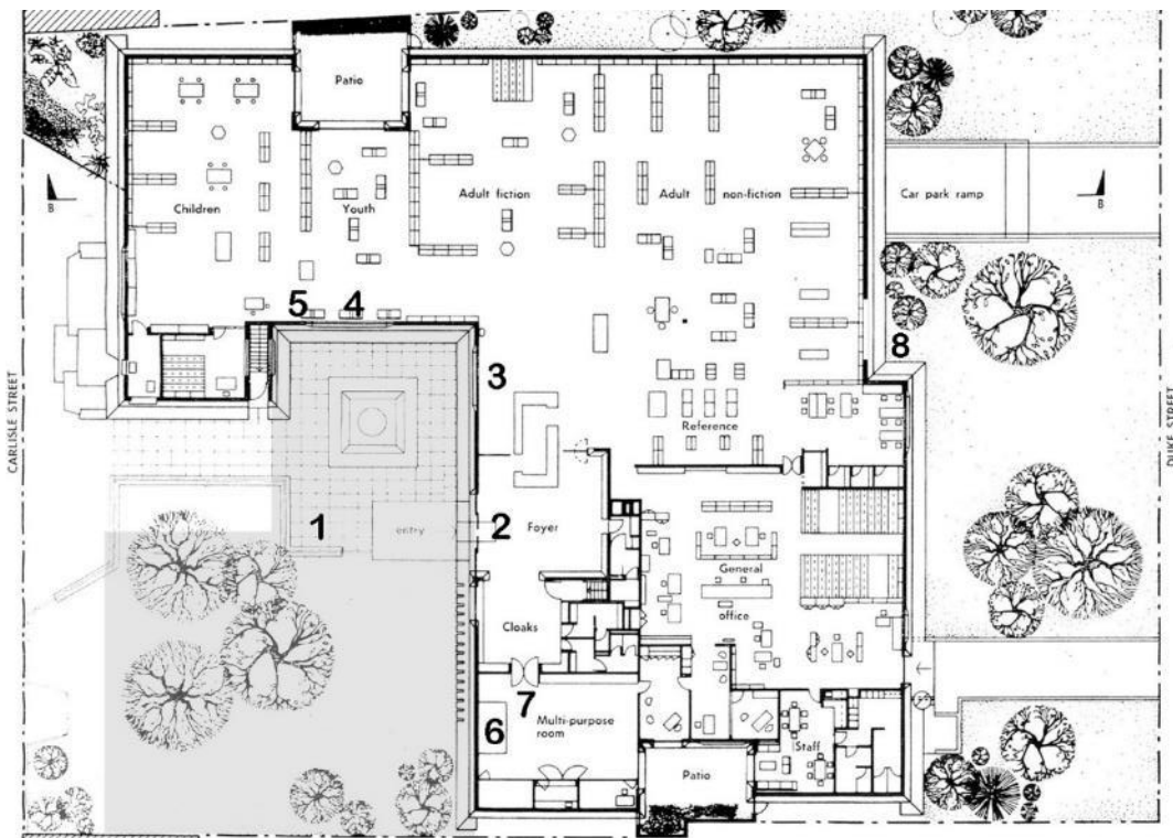
Figure 11 (1) Indicates the extent of the addition to the original library completed in 1993; (2) the location of the original entry and sidelights; (3) window sill that was demolished for a full-height opening; (4) glazing removed from opening; (5) new full height opening; (6) new double door opening; (7) opening infilled; (8) window to the north wall of the reading room (north is at right)
