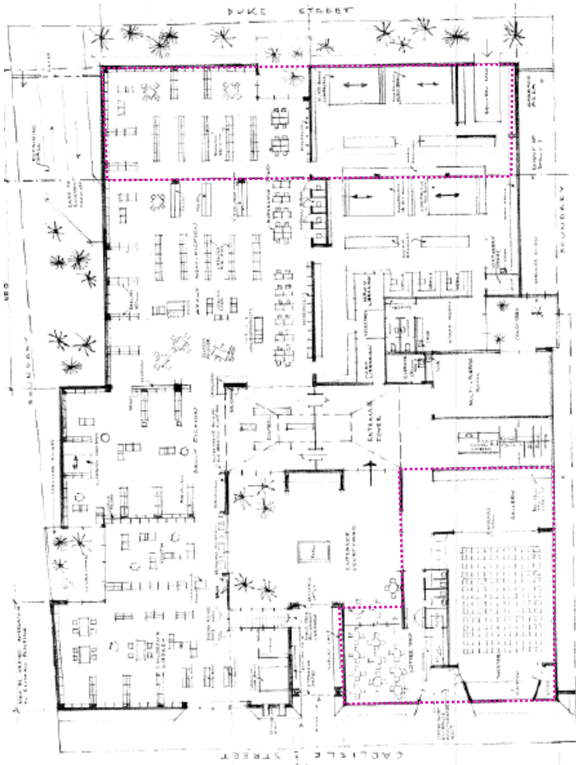
Figure 4 Sketch plan of Stage 2 by Enrico Taglietti, 1971, with the alterations indicated: a theatre and café were proposed at the south-east of the plan and the building was extended to Duke Street: north is at top Source: Enrico Taglietti
