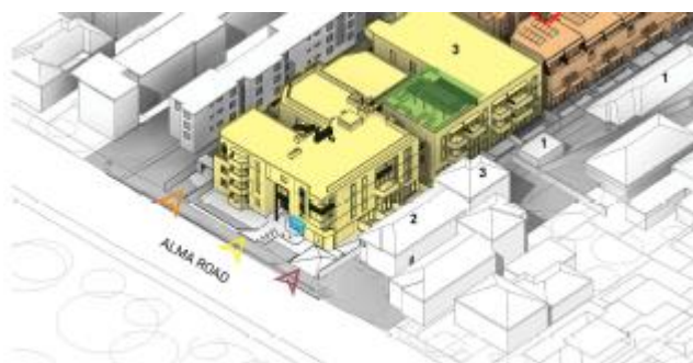
Figure 7: 3D of northwest corner showing proposal in context of adjoining front setbacks (TP000 dated 27.07.2023)
