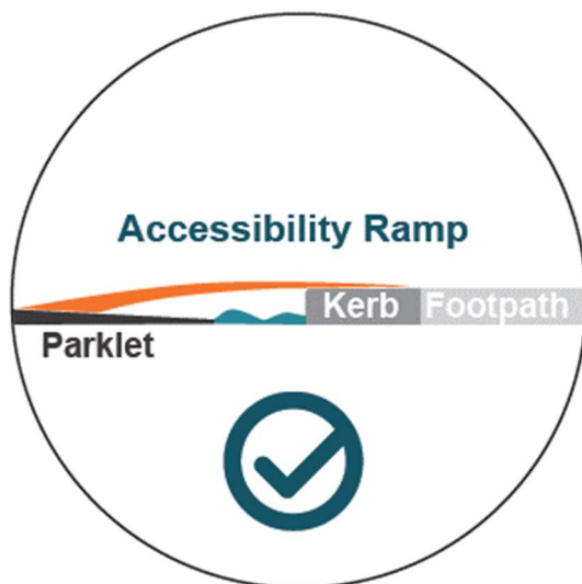
Figure 18: Seasonal Business Parklets are not required to have a platform that is level with the footpath and may therefore use a ramp onto the carriageway.
