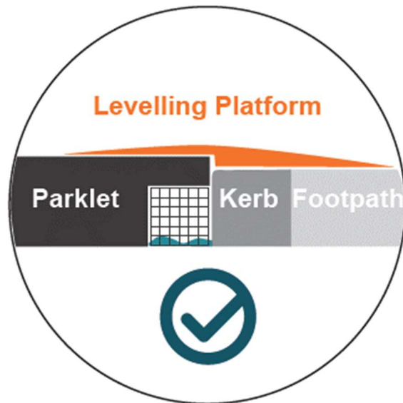
Figure 20: Levelling platform creates a smooth transition and prevents tripping hazards
