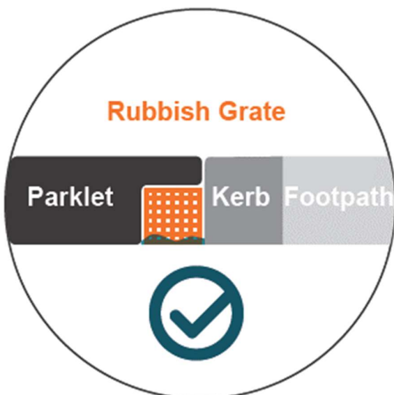
Figure 26: A rubbish grate will prevent litter from being trapped under the platform
